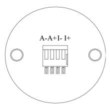
If the axle is kitted out of a plug ( LUMBERG), connectors are marked as following :
